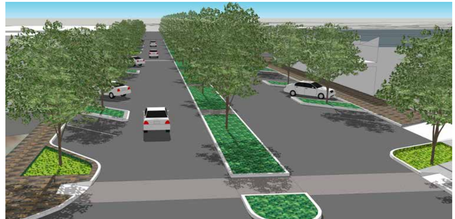
Porter Street vision - 3m treed median and verge planting create a boulevard effect. Rain gardens in the foreground collect, slow and treat stormwater.
