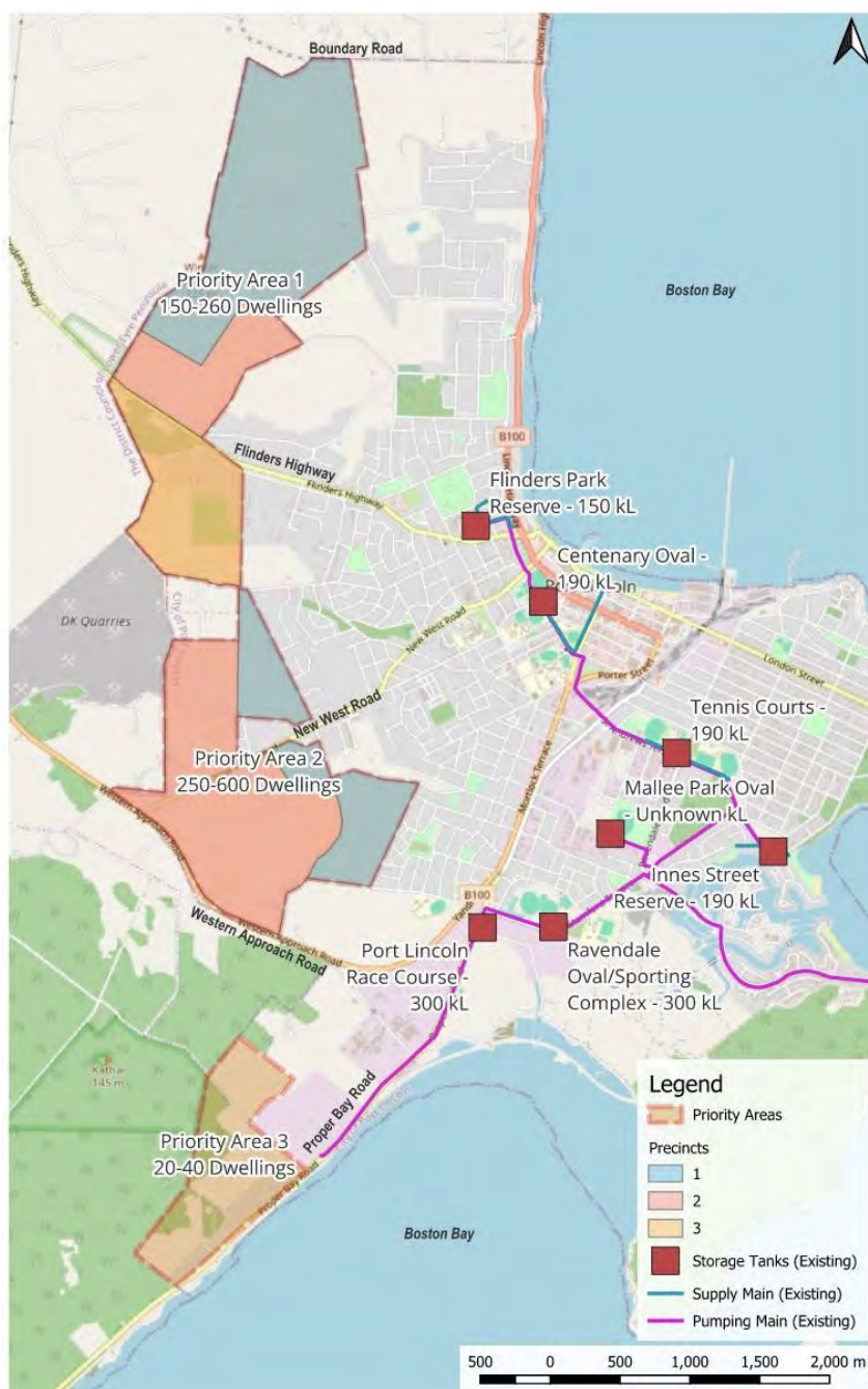
Figure 10-1: Council's Recycled Water Network
