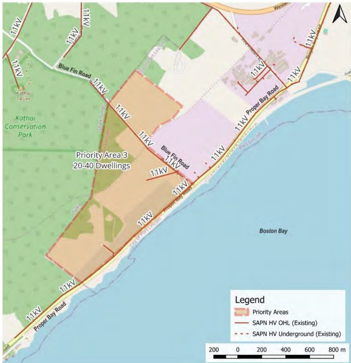
Figure 8-3: Existing Electrical Infrastructure - Priority Area 3
