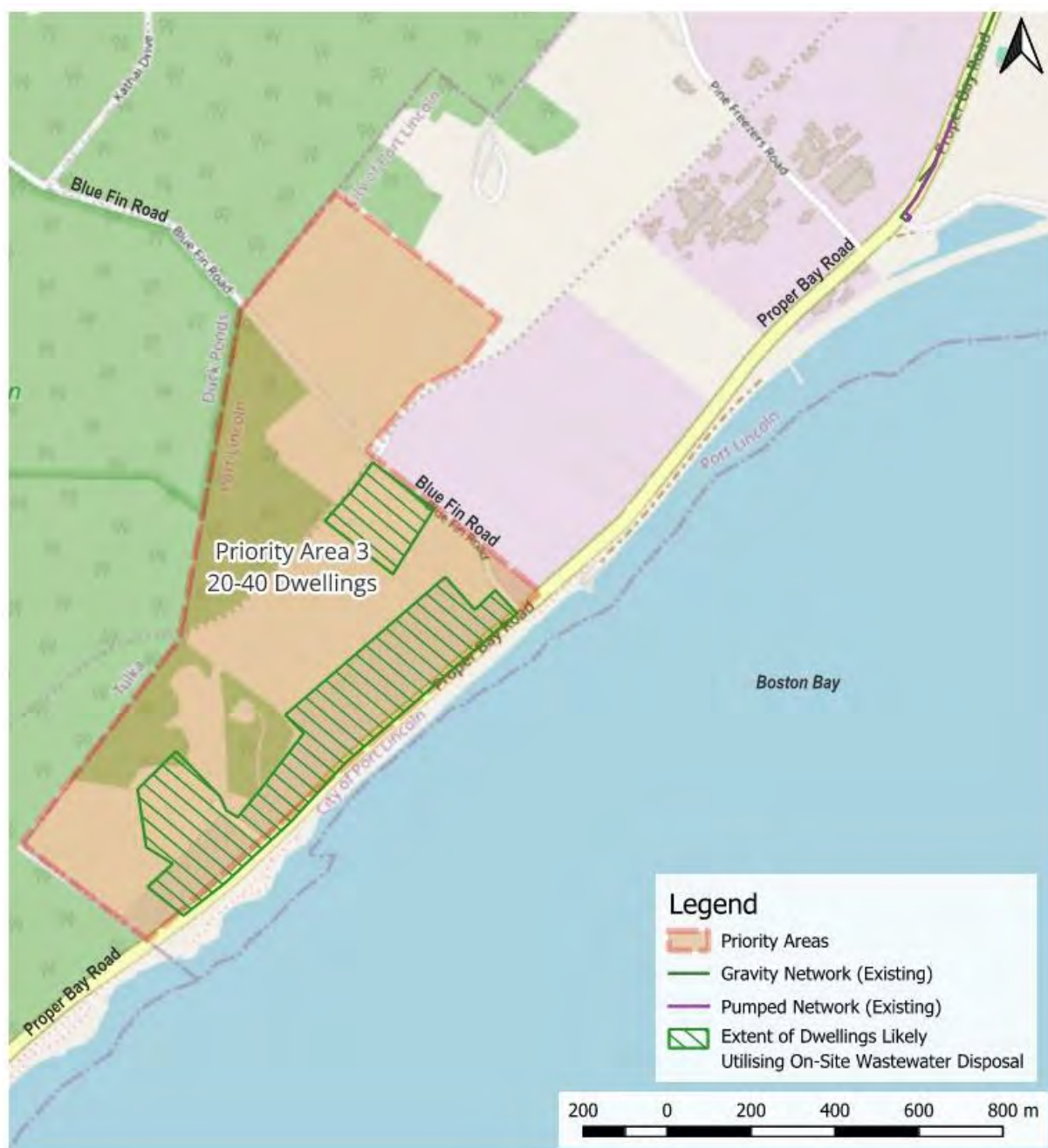
Figure 6-3: Existing SA Water Infrastructure – Priority Area 3
